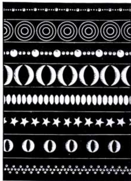
Fig. 7 (in order downwards). Showing the timbre of different sounds: xylophone, electric bell, two-note bell, bassoon, flute, an instrument rich in upper harmonics, bassoon and various high pitched sounds.
