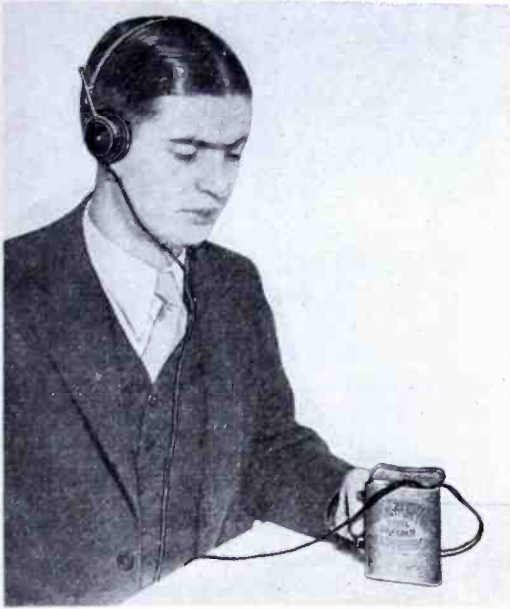
The tobacco can crystal receiver in operation. The man is shown adjusting the knob of the tuning condenser
